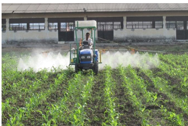
Figure 2. Field evaluation of developed “Small tractor operated boom sprayer”
