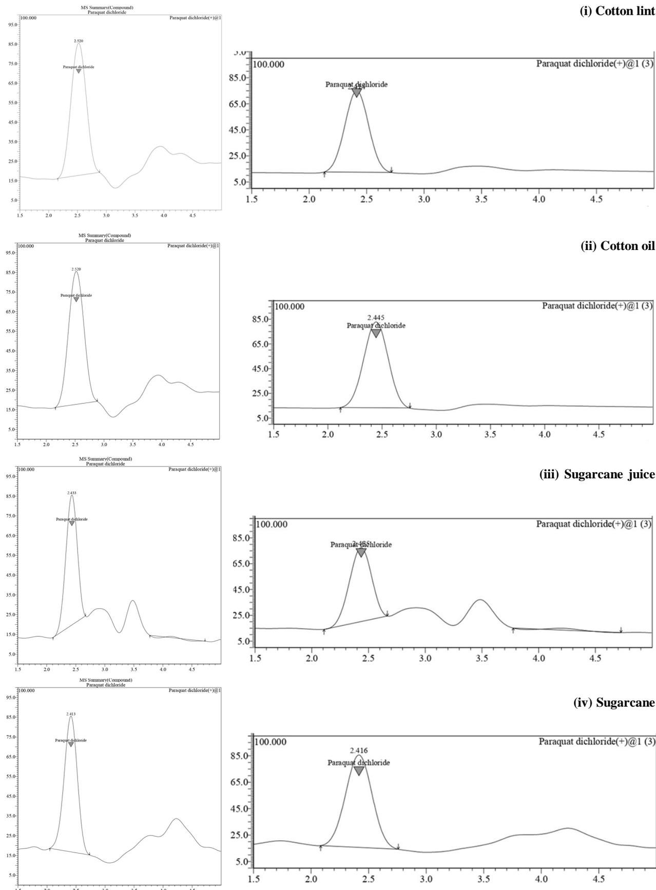
**Figure 2. Chromatogram of matrix match standard (left) and recovery at LOQ level (right) for selected matrices in cotton and sugarcane by LCMS**
