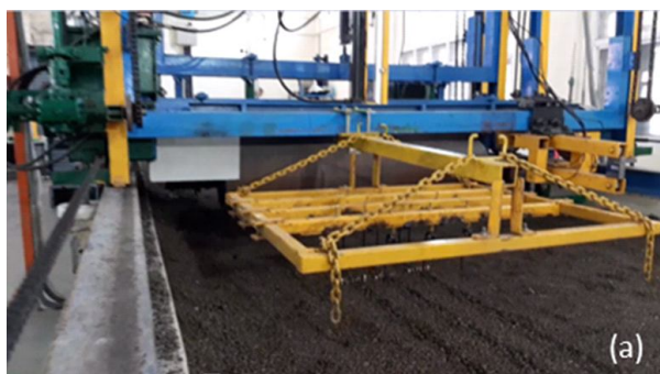
Figure 1. Experimental setup for soil bin study of garlic weeder (a) laboratory model weeder (b) soil bin
