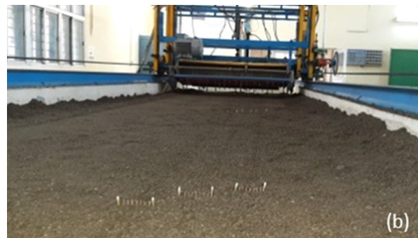
Figure 1. Experimental setup for soil bin study of garlic weeder (a) laboratory model weeder (b) soil bin
