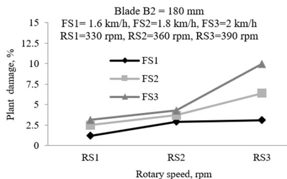
**Figure 5. Influence of blade length, rotor speed and forward speed on crop plant damage during the operation of two rows self-propelled narrow crop rotary weeder**
