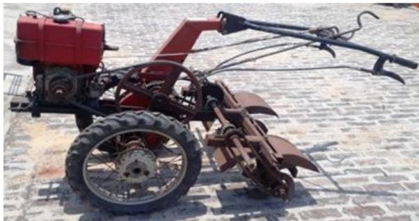
Figure 1. Two rows self-propelled narrow crop rotary weeder
