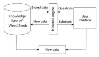
Fig. 1. KBS Design Architecture
