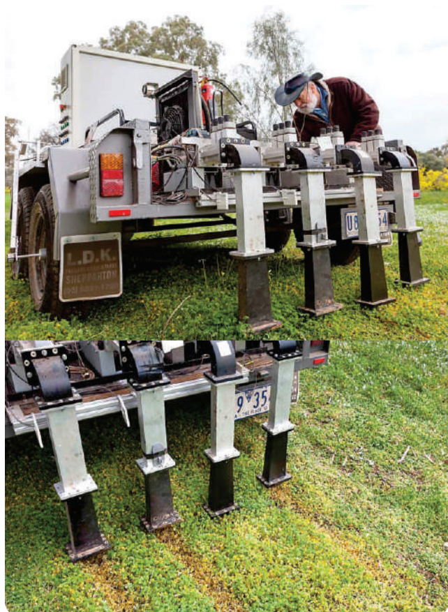
Figure 16. Microwave weeder (Source: Courtney 2021)
