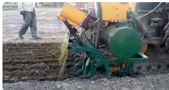
Figure 1. Lucky seed drill does sow rice seeds and spray pre-emergence herbicide simultaneously and provide adequate control of first flush of weeds
