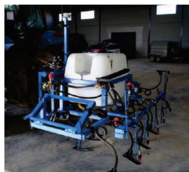
Figure 11. Row-centering RTK-GPS based cultivator cum band sprayer
