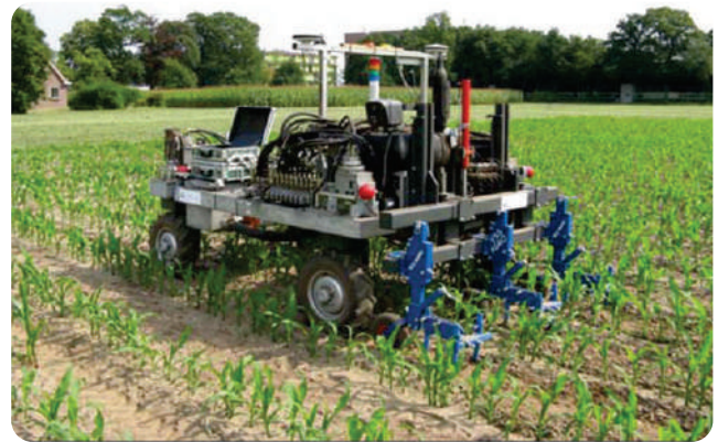
Figure 14. Autonomus RTK-GPS based weeding robot (Source: Bakker et al. 2010)
