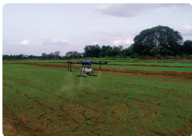
Figure 2. Spraying of early post-emergence herbicides by drones at Tamil Nadu Agricultural University, Bhavanisagar
