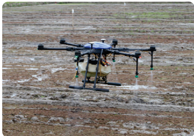
Figure 1. Spraying of pre-emergence herbicides by drones, Tamil Nadu Agricultural University, Coimbatore
