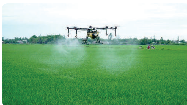
Figure 10. Herbicide application through drone (Source: Anonymous 2020)
