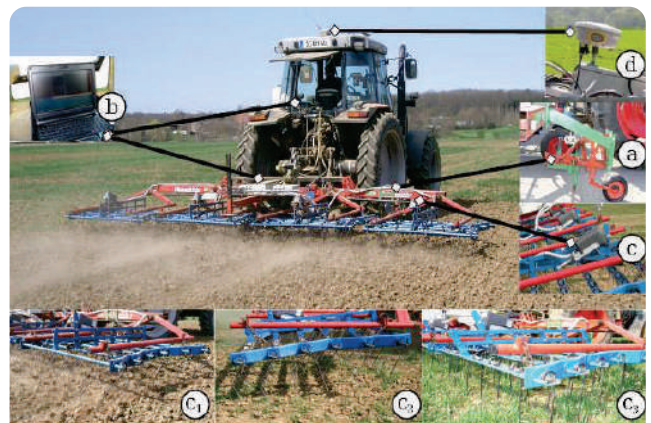
Figure 14. Autonomus RTK-GPS based weeding robot (Source: Bakker et al. 2010)
