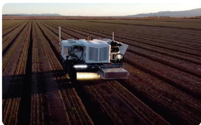
Figure 17. Laser beam based autonomous weeder robot (Source: Lavars 2021)
