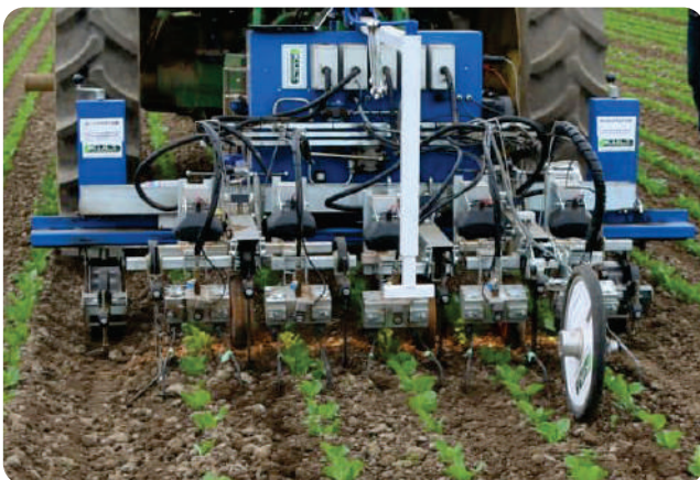
Figure 13. Machine vision based online weeding (Source: Anonymous 2018)
