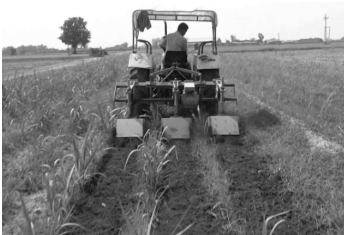
Figure 10. Rotary weeders (source: www.Mygreen.Farm ; CoEFM, Ludhiana, India)
