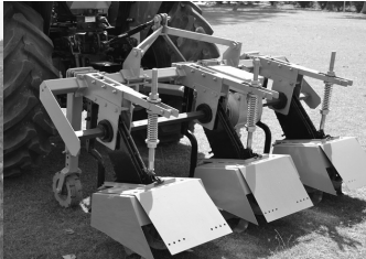
Figure 10. Rotary weeders (source: www.Mygreen.Farm ; CoEFM, Ludhiana, India)
