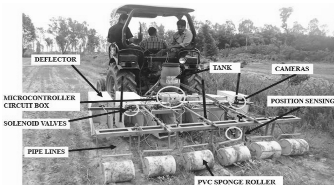
Figure 27. On-the-go position sensing and controller predicated contact-type weed eradicator
