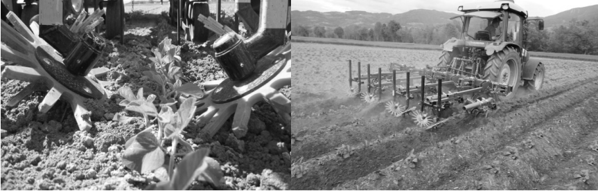
Figure 12. Finger weeder (source: Thomas Hatzenbichler Agro-Technik GmbH, Andrä, Austria)
