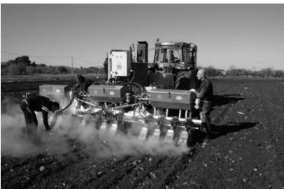
Figure 18. Soil steaming (source: Peruzi et al. 2018)
