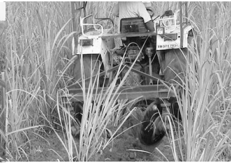
Figure 11. Earthing up cum ridging type weeders (source: Ramakumar Industries, Tamil Nadu, India)
