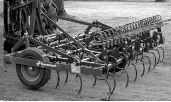
Figure 7. Tyne harrow (source: https://cy.wiktionary.org/wiki/oged )
