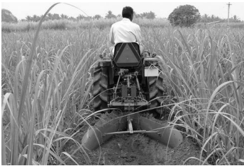
Figure 11. Earthing up cum ridging type weeders (source: Ramakumar Industries, Tamil Nadu, India)
