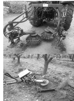
Figure 14. Brush weeder (source: NaturaGriff, France)
