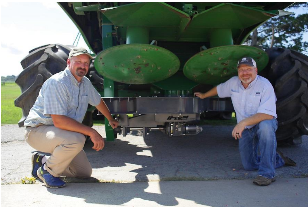
Photo: Jason Norsworthy (left) and Tom Barber with the new Integrated Harrington Seed Destructor being evaluated in Arkansas. (Photo from University of Arkansas)
