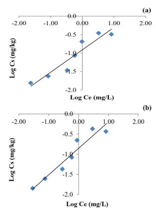
Figure 2. Linear plots of freundlich isotherm for tembotrione adsorption in maize soil after 12 h of equilibrium (a. tembotrione alone; b. tembotrione +isoxadifenethy)
