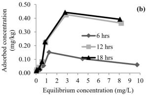
Figure 1. Tembotrione adsorption in maize soil revealed by batch equilibrium experiment (a. tembotrione alone; b. tembotrione +isoxadifenethy)
